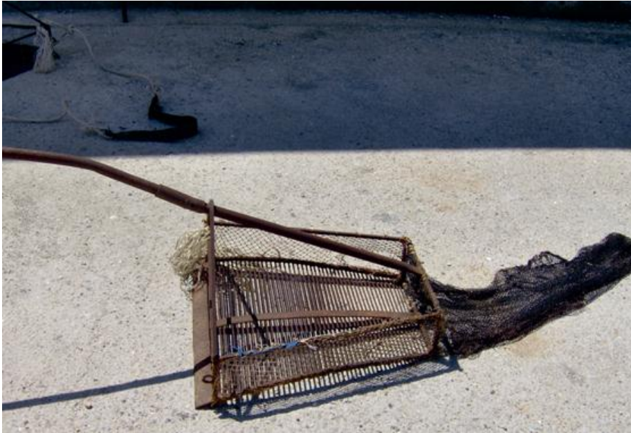
Figure 5. Hand dredge used to harvest wedge clam ( Donax trunculus ).
